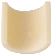
DEGUSSIT AL23 sample after the corrosion test described below. The absence of methylene blue staining indicates that sulphuric acid did not corrode the microstructure.
